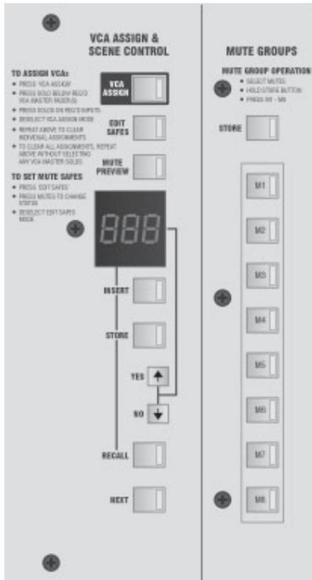
Used to scroll through the scenes. Holding down the keys will gradually scroll faster (auto-scroll). Pressing ↑/↓ while Recall is being held down will scroll the scene and recall it, but not if the display is auto-scrolling. The YES/NO facility is used to confirm or cancel Store or Insert actions.
