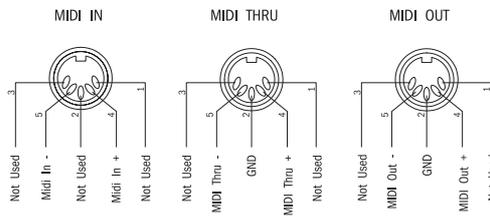
The MIDI IN signal is buffered by an opto-isolator.
